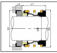
Rubber-bellow seals with boot mounted stationaries and Stainless Steel spacer-rings, to suit internal dimensions of Ebara® "EVM" and "EVMW" vertical multi-stage pumps.
