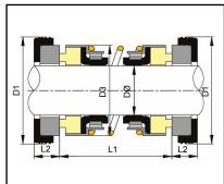
Rubber diaphragm double-ended seals with boot mounted stationaries, to suit the internal dimensions of Ebara® "Best-", "Right-" and "DW-" series, small submersible pumps. This common seal STK is also utilised by other pump manufacturers for small portable submersible pumps.
