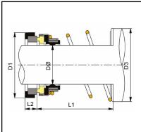
Stramek manufacture and stock a variety of standard range seals to suit various Eureka® pumps (now part of Hamworthy®, formerly Thune-Eureka®). STK 277 is an elastomer diaphragm seal, with reverse taper seal to specifically suit the "CG-" series centrifugal pumps, widely used in marine applications.
