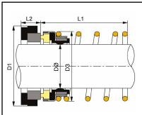
Elastomer diaphragm seals to 2.3/8" shaft size, with extended taper coil, to suit internal dimensions of Eureka® "CAC, CAV and CAX-" series centrifugal pumps, widely used in marine applications.
