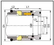
Stramek manufacture and stock two sizes of hydraulically balanced, multi-spring hygienic seals to suit Variflow® KN-series pumps, directly replacing the original design.
