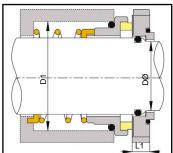
Stramek manufacture and stock a range of singlespring stationary seals, with Stainless Steel counterring rotaries with outer turning-vane, and inserted Carbon sprung-stationaries.
