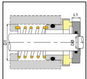
Stramek manufacture and stock a range of singlespring stationary seals, with Silicon Carbide faced counter-ring rotaries, and inserted Carbon sprungstationaries to replace the chrome-oxide coated rotaries of the O.E.M. seals.
